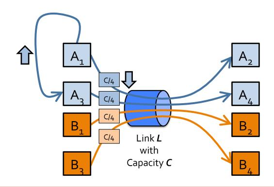
To maintain proportionality, equal amount of traffic must be moved from A1-A2 to A1-A3 => **Underutilization of A1-A3**
