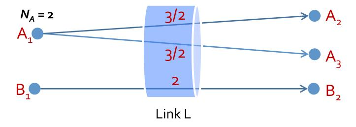
To generalize, weight of a flow A-B on link L is  $W_{A-B} = \frac{W_A}{N_A} + \frac{W_B}{N_B}$
